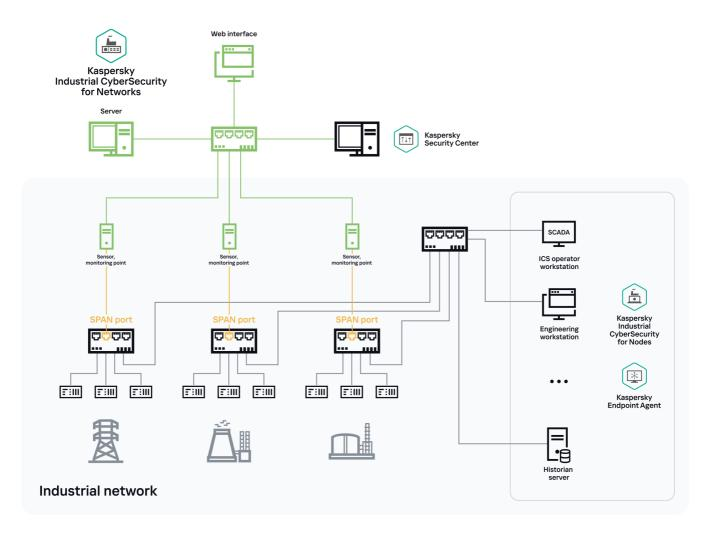
Example deployment of a Server and three sensors
