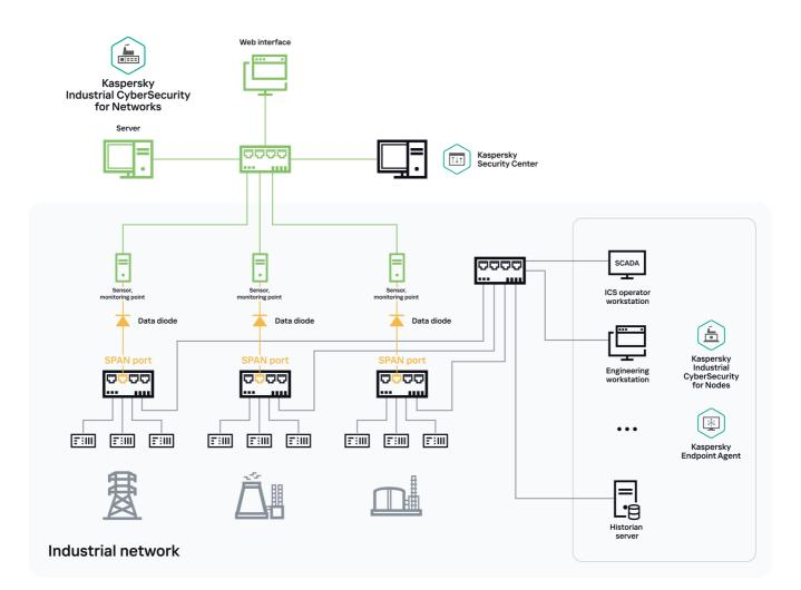
Example connection of sensors via data diodes
