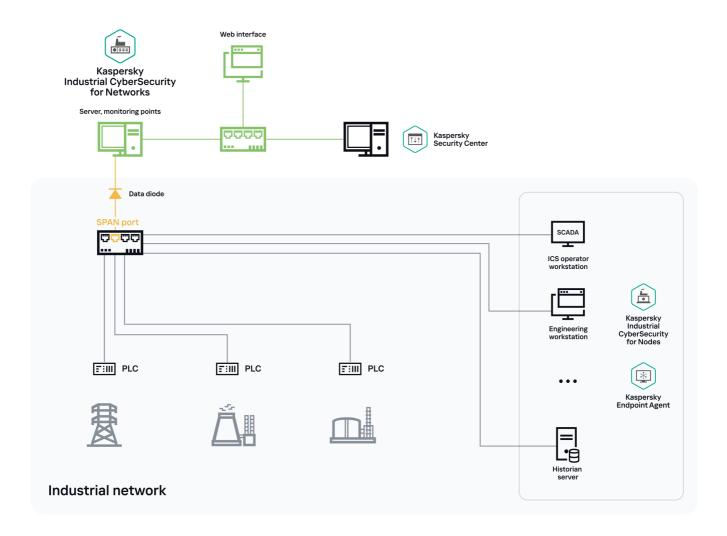
Example Server connection via data diode
