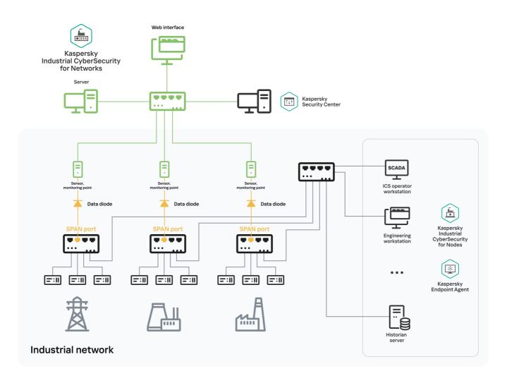
Example connection of sensors via data diodes
