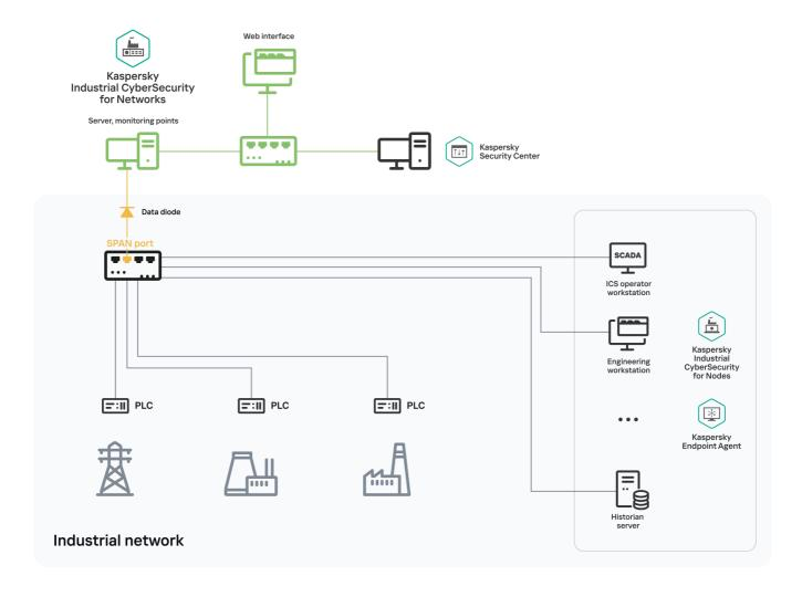
Example Server connection via data diode
