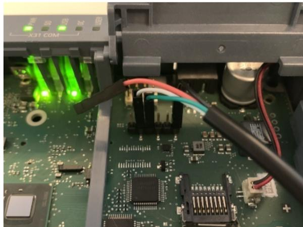
Example of connecting a USB-UART cable to a UART diagnostic connector
